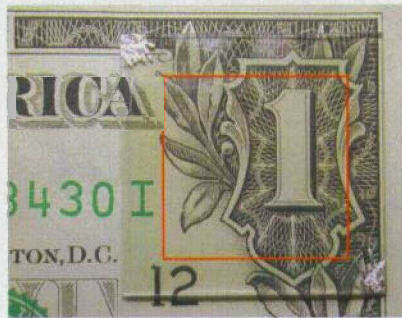
Photo 1—Spin-coated ZnO TFTs. 56 patterned ZnO TFTs and 24 contact resistance test structures are present inside the red box.
